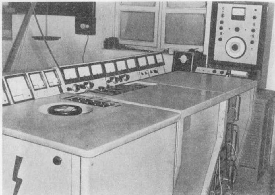
Figure 7. Control desk on test bench used for chain vibration measurement
