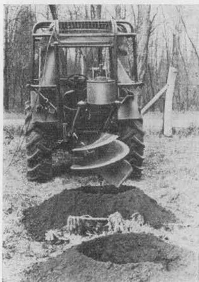
Figure 2. Planting holes and earth deposition carried out by the "ERTI" auger
