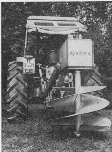
Figure 1. The newest, model-designed type of the "ERTI" planting auger
